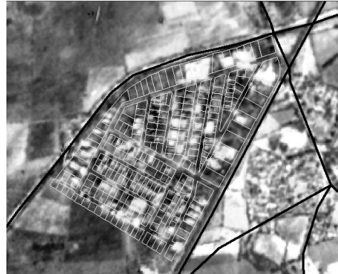
Fig: 3 Digitized layout map of Viramgam GIDC estate overlaid on satellite imagery
